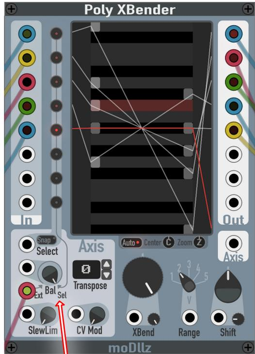
Axis can be balanced (with Knob or CV) between Selected (from inputs) and External (from dedicated input)
