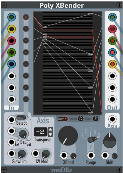
Example of XBending to negative value (5v Range). The outputs diverge from the Axis (input 3)
