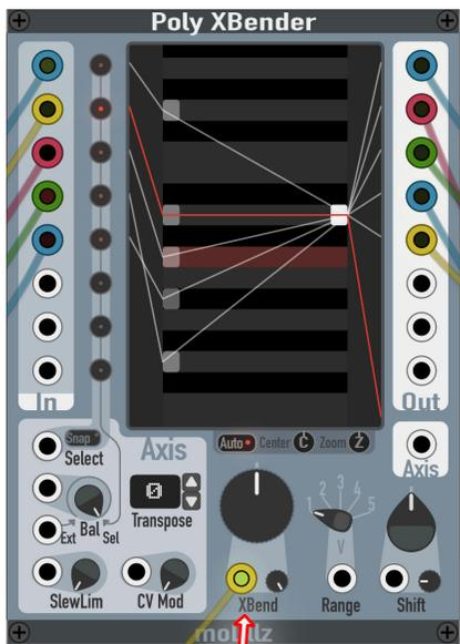
5v cv applied to the XBend, with 1v Range. All output signals match the Axis (Input 1). CV input is 24 step-trimmed
