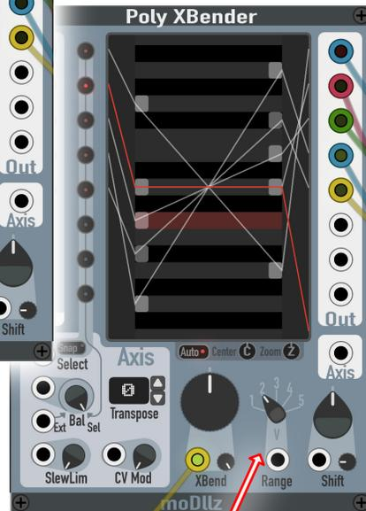
XBend Range increased to 2v. The output signals diverge from the Axis, ending up "mirrored" from their inputs
