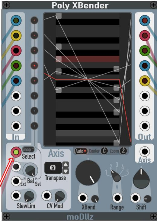
Axis can be selected from CV continuously (crossfading inputs) or snapped to inputs
