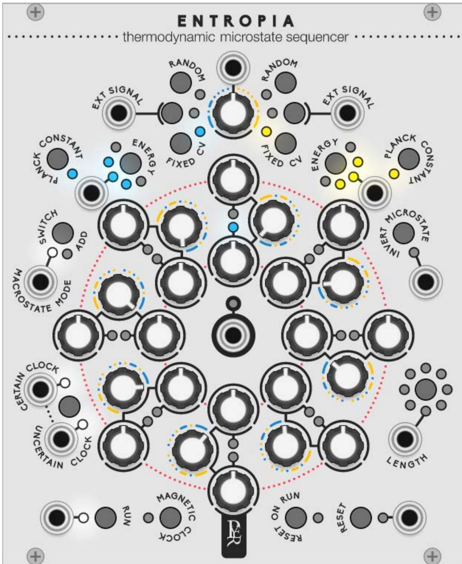
With 3 sources for both sequences and two blend modes there are 18 different ways to use the sequencer.
