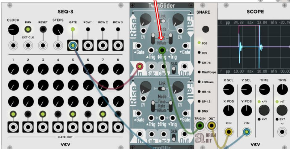
Generate Gates from Trigger (Trigger Input : with Rise (or Fall) time > Rise (or Fall) Gate Out)
