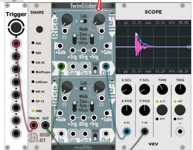
Generate Trigger signals at the beginning and ending of a Gate :
