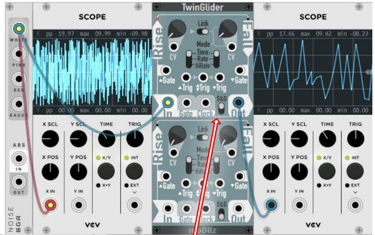
Get "slow" noise signals for random modulation (noise Input : Sample &Glide on)
