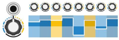
When the offset knob is turned in the yellow direction, it adds an offset to the yellow direction for every step.
