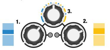
All the blue knobs and the yellow knobs determine a **blue and a yellow sequence**. The position of the state selector will define the probability to play the blue value, or the yellow one. The resulting sequence is the **macrostate**.
