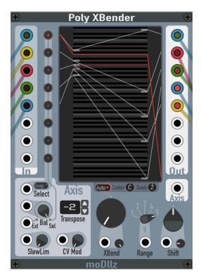
Example of XBending to negative value (5v Range). The outputs diverge from the Axis (input 3)
