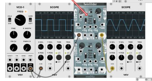
Get "slow" noise signals for random modulation (noise Input : Sample & Glide on)
