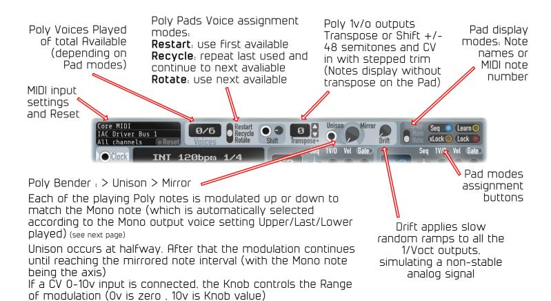
Poly Bender example: Here's a chord (E3 G#3 A3 C#4) processed with the Poly Bender, with different Mono settings. At half way all notes match the Mono note. Then they continue up/down until the mirrored chord
