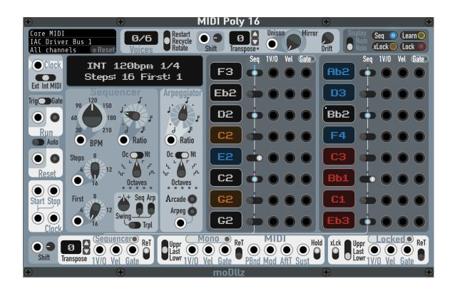
The incoming MIDI notes are dynamically assigned to 16 "Pads", with independent 1V/Oct, velocity and gate outputs each.
