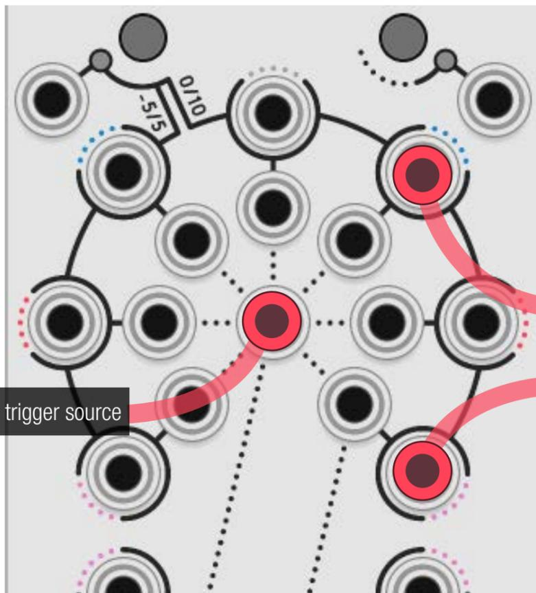
When a trigger is connected, the outputs use the trigger to sample and hold their internal noise generator and send random CV.
