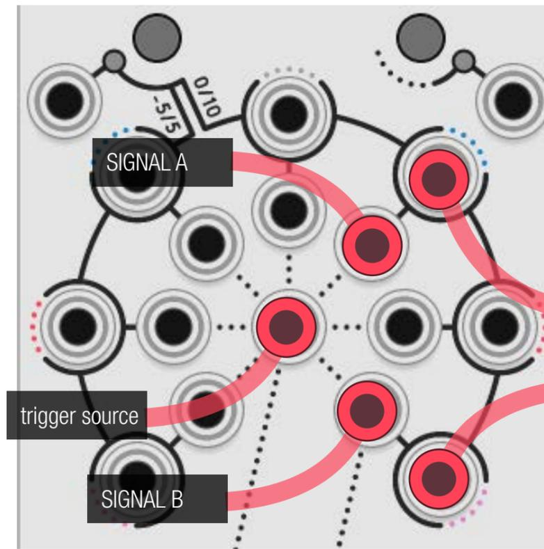
When a trigger and an input are connected, the noise generator is bypassed, and the S&H uses the input as material.
