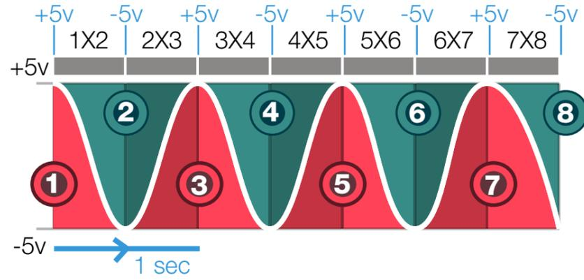
**A triangle wave** will make linear crossfade, while a **sine wave** will create an exponential cross-fade
