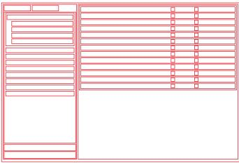
For example the Introjucer window can be broken down into a series of nested children Components (shown in red).
