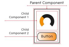
Components allow us to build complex, hierarchical and responsive interfaces for different devices and screen sizes, whilst keeping the code-base clean, modular and maintainable.
